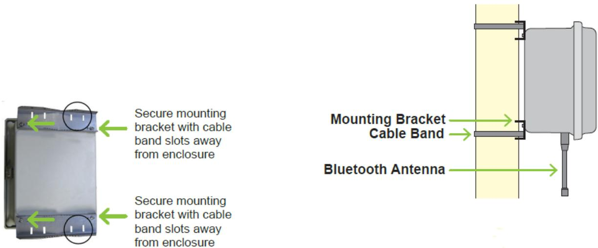
d. Align the Enclosure—as shown below:
