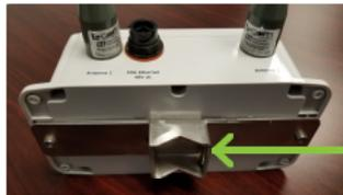
Mounting Bracket slots for up to 1-inch metal banding.
