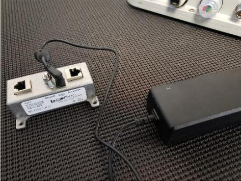
7. Connect the RSU to the Data+PWR port of the POE Injector with an Ethernet cable. The RSU Power LED indicator should light up with power.
