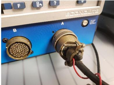
2. Plug the “A” power cable into an AC power source. The controller should power ON.
