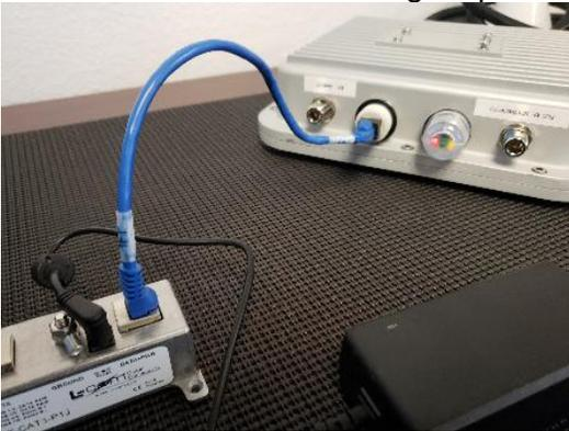
8. Connect the POE Injector Data port to Port 1 of ENET-1 (WAN) of the controller with an Ethernet cable.
