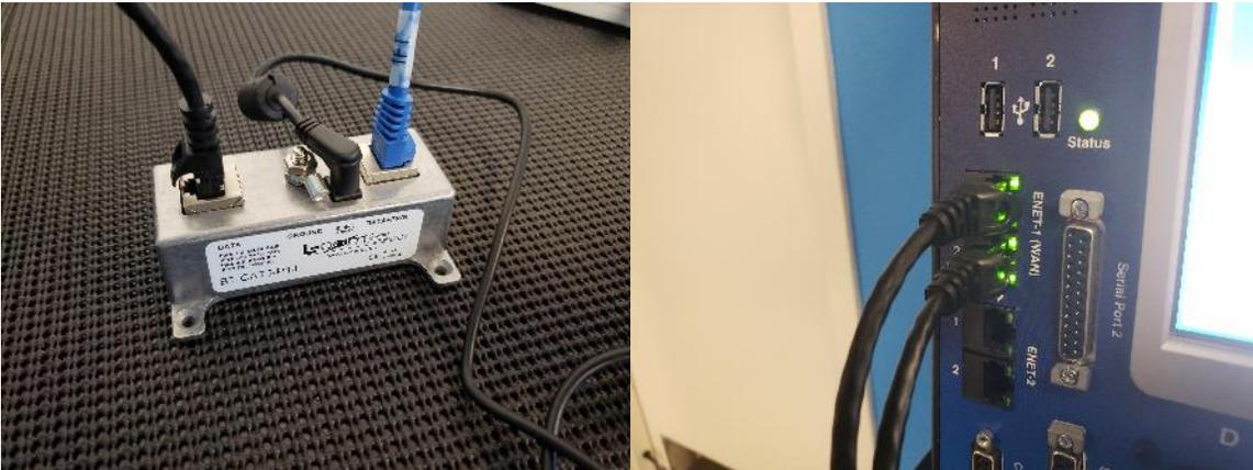
9. Connect the computer to Port 2 of ENET-1 (WAN) of the controller with an Ethernet cable.
