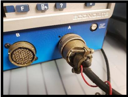
1. Attach the Traffic Controller “A” power cable to the “A” connector of the controller.
