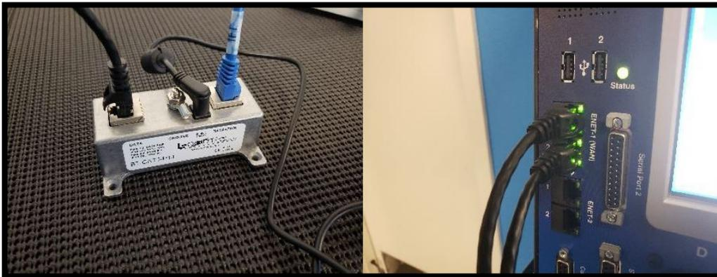
9. Connect the computer to Port 2 of ENET-1 (WAN) of the controller with an Ethernet cable.
