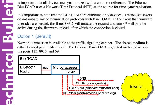
Ethernet BlueTOAD uses port 123 to access the north-america.pool.ntp.org time server. Port 8010 is used to transport the collect MAC addresses and their respective time stamps. Port 69 is used for firmware upgrades (as needed). It is important that a valid DNS address is used such that the domain name can be recognized.
